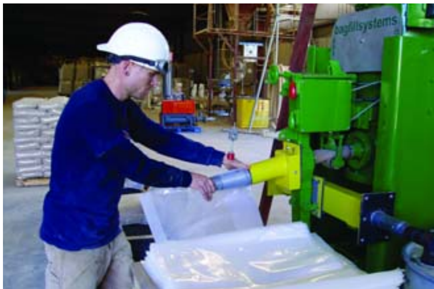
An operator slides the self-sealing valve bag's opening over the dustless bag-filling system's nozzle.
