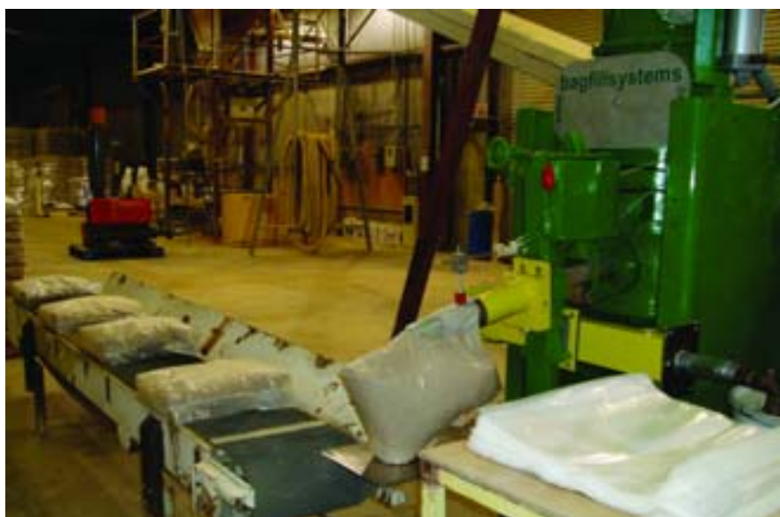
The mechanical scale supports the bag as the air packer fills it, minimizing the need for operator assistance.
